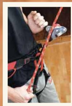
When using a GriGri, the braking hand must never let go of the braking rope.
