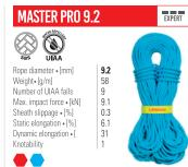
This rope defeats the stigma that thin ropes aren't durable. You don't need to carry one rope for practicing and another one for redocint. Innovated, extremely fine SBS sheath significantly prolongs its lifespan. The rope is at the same time soft enough and easy to work with.
