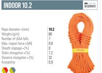
A rope with braided core developed especially for top-rope climbing at gyms. Suitable for climbing schools and rentals
